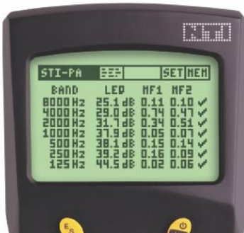
Acoustilyzer AL1 STI-PA test results with modulation indices
